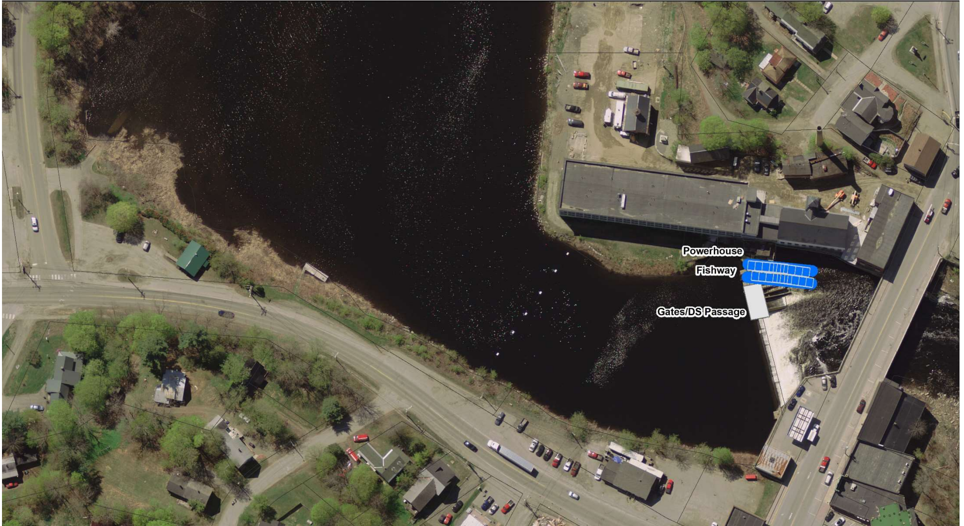
Figure 1. General location sketch for options HP 1 and HP 2 (Restore Power Generation, Retain Dam, Maintain Impoundment at Current Levels, Technical Fishways). Actual configuration, orientation, scale and size will vary pending additional development.
