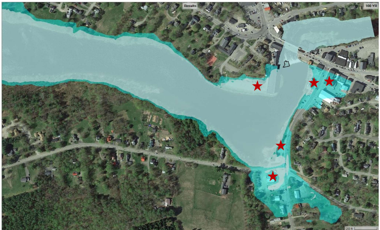
Figure 8. Aerial comparison of simulated flood resilience benefits for the 100-year return period flood for the Dam Removal strategy (Removal-gray) to existing conditions (cyan).
