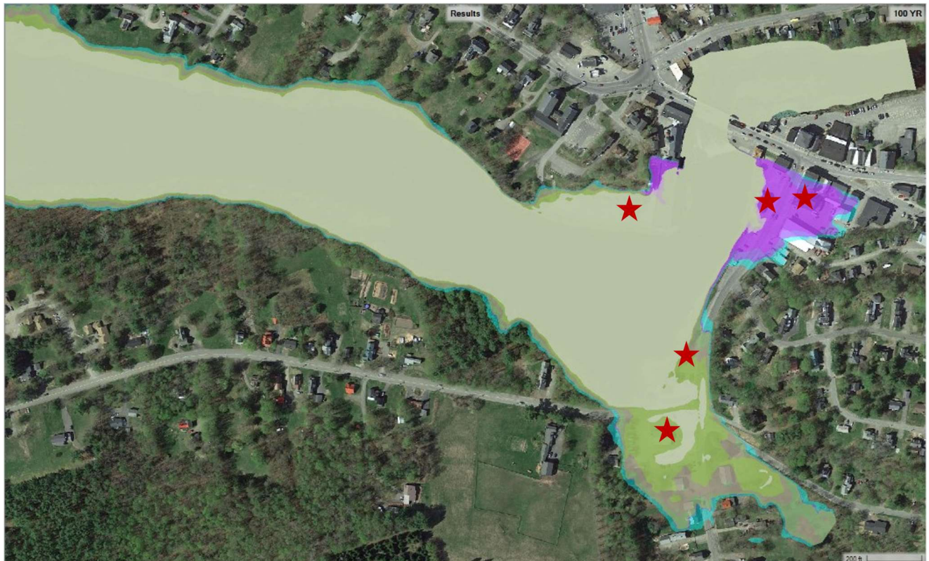
Figure 10. Aerial comparison of simulated flood resilience benefits for the 100-year return period flood for the five alternatives detailed in Section 0. The alternatives (M1-purple, L1-lavender, N6-olive, N7-brown, N6-green, R1/R1-light green) are compared to existing conditions (cyan)
